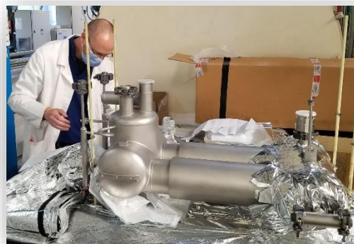
Figure 2: Outside view of the heat exchanger before testing at 1.8 K.
